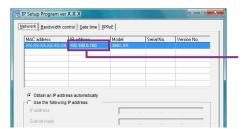
When the IP address set (or set automatically) is displayed in the IP address column, the IP address of the camera has been assigned correctly.
